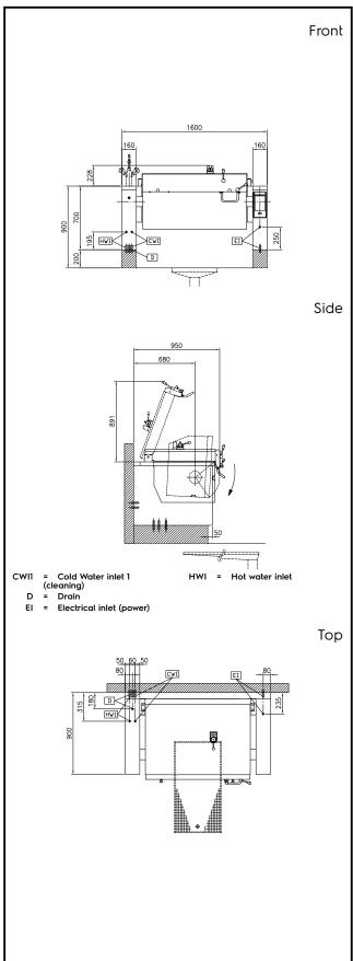
Electric Supply voltage: 400 V/3N ph/50/60 Hz Total Watts: 20.6 kW Installation: FS on concrete base;FS on feet;On base;Standing Type of installation: against wall
